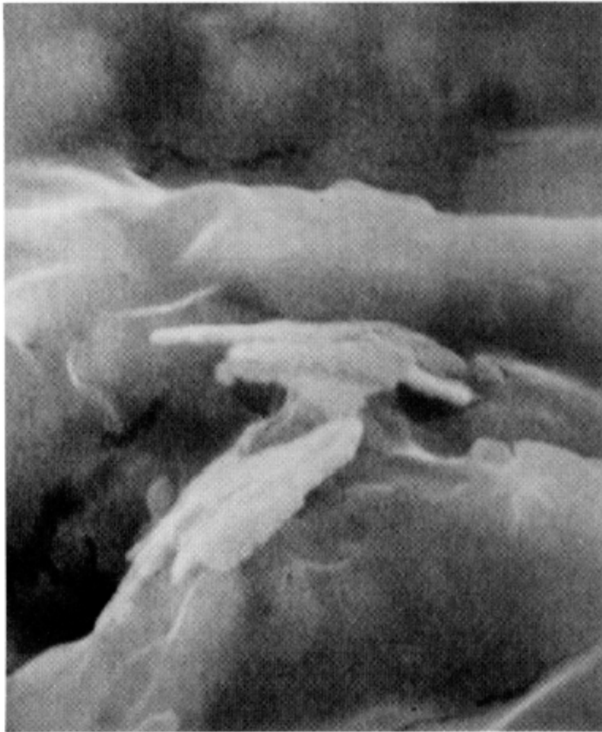
FIGURE 3. Wafer-like platelets on top of a crest on the external surface of polyurethane catheter ( \times 10,000 ).
